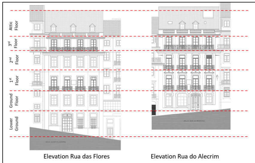
Figure 28 – Floor identification (Architect Drawings adapted)
