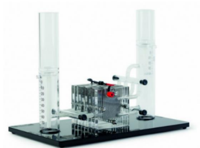
Figure 19 -E207 PEM Electrolyzer
