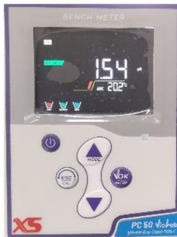
Figure 22 -Water conductivity test
