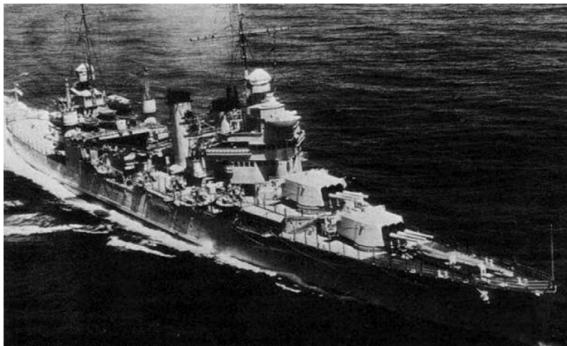
Figure 13 – The New Orleans class were the final version of the U.S. “Treaty” cruisers to be built in numbers. Like all Treaty cruisers they were a compromised design, the U.S. Navy renouncing torpedo armament but adopting a powerful AA battery. Three of the class Vincennes, Quincy and Astoria were sunk by gunfire and torpedoes of Japanese heavy cruisers in a single battle (Savo island) during the Guadalcanal campaign
