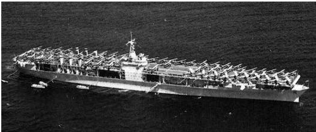
Figure 7 – The USS Ranger, the first U.S. purpose built carrier, shows the U.S. Navy early emphasis on a large air group and an (semi) open hangar for ease of air operations 21 .
