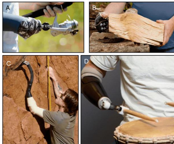
Figure 6 - Activity-specific prosthesis (A) for fishing (B) for work with wood (C) for climbing (D) for playing drums [23].
