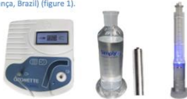
Figure 1 – Ozone generator machine; Ozone water bubbler system; Microbubble water ozonation column
