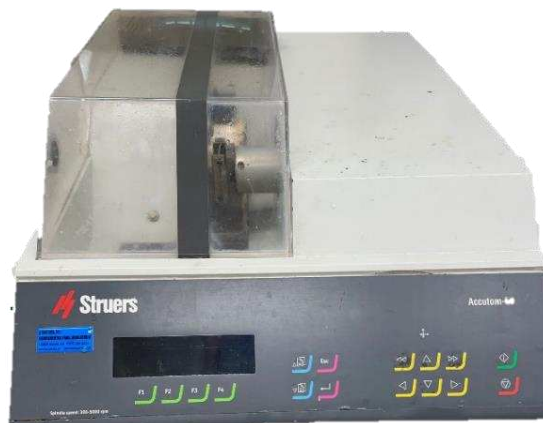
Figura 2. Micrótomo de tecidos duros (Accutom-50, Struers A/S, Ballerup, Denmark)
