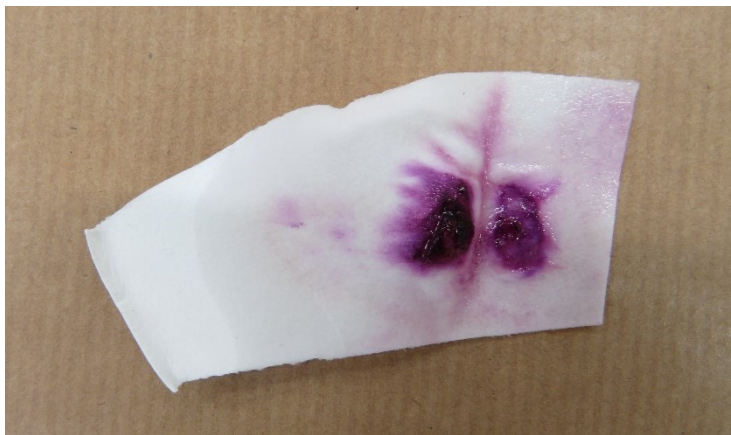
Figure 10 - Photograph taken during this study representative of a positive Acid Phosphatase test.
