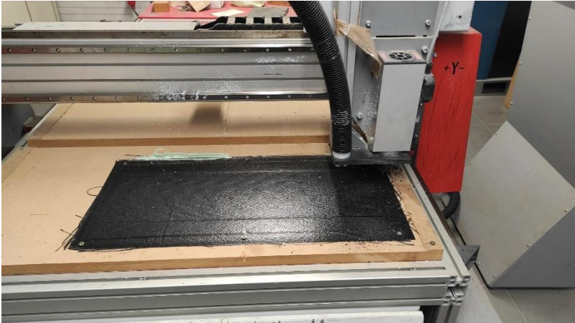
Figure 23 - Laminate ready to be cut in the CNC machine.
