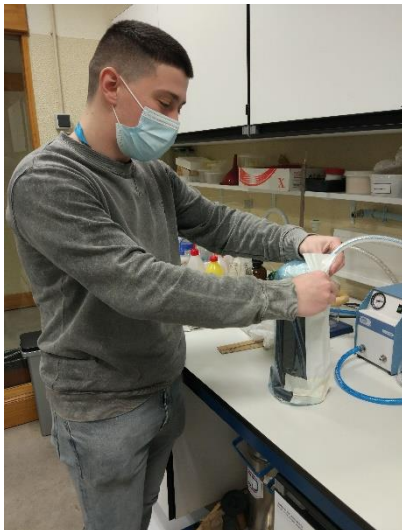
Figure 30 - Air being removed from the plastic bag.
