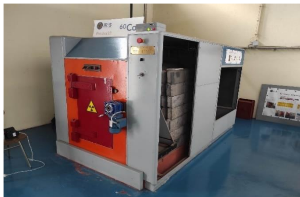
Figure 27 - Precisa 22 cobalt-60 gamma irradiator.
