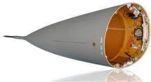
Figure 3 - F16 Radome (General Dynamics to Build Wide-Band Radomes for F-16s | Shephard, n.d.).
