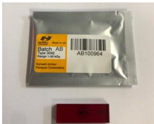
Figure 17 - PMMA routine dosimeter (Harwell Amber Perspex Dosimeter) (Soares, 2021).
