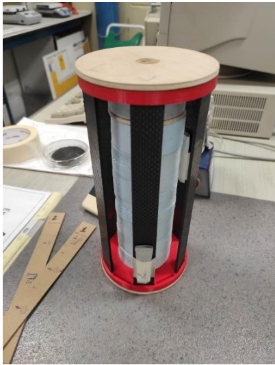
Figure 28 - Irradiation supports designed by Soares (2021).
