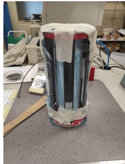
Figure 31 - Irradiation support sealed in the vacuum bag.
