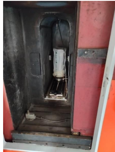
Figure 29 - Irradiation support inside irradiator chamber.
