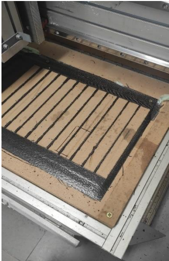
Figure 24 - Laminate after cut and with the test specimens removed.
