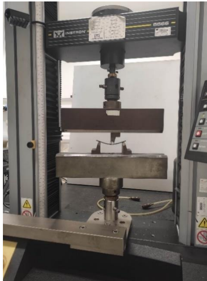
Figure 38 - Instron model 5566 with a 500 N load cell installed.
