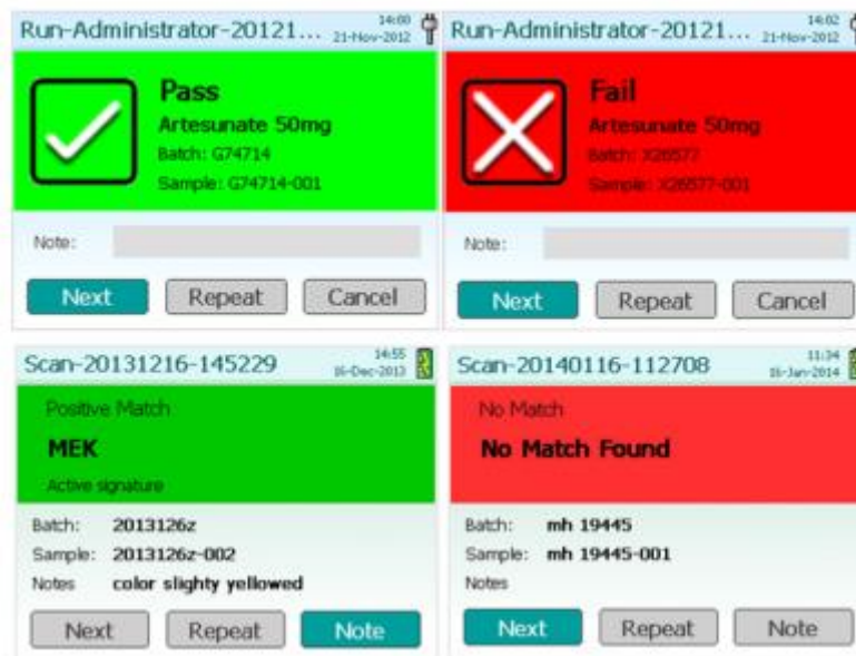
Figure 9 - Example of both the "Pass" and "Fail" screen and respective match using the TruScan RM [39].
