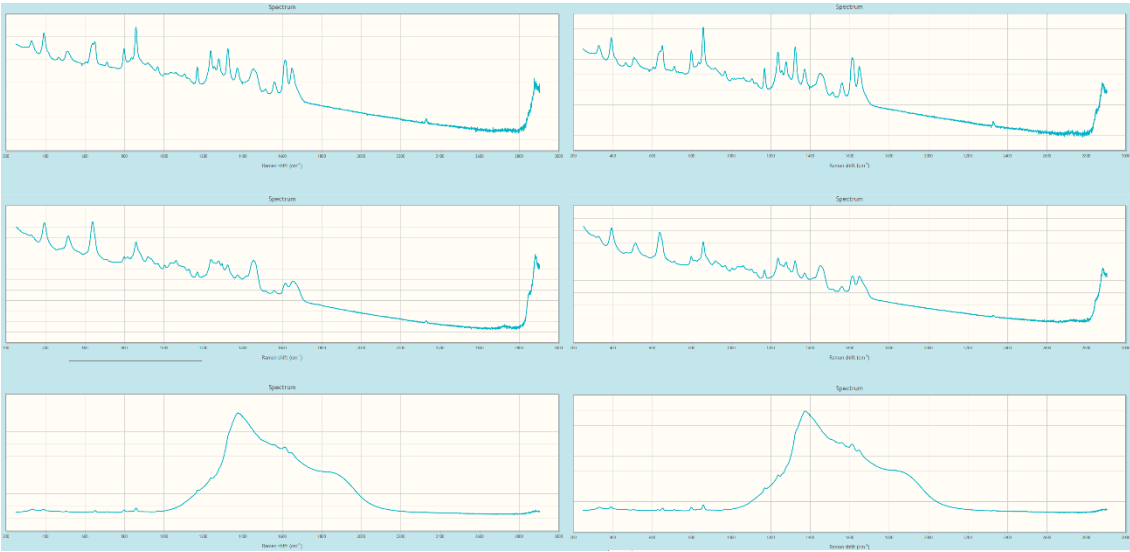
Figure 22 - Raman spectra of two different batches of component E (one left and the other right). On top readings with PnN in full capsule, in the middle readings with PnC in full capsule and readings of content in vial below.
