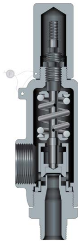
Figura 10 – Exemplo esquemático de válvula de alívio ( https://www.cw-valvegroup.com/sites/default/files/Library/CW_2700Catalog_R9-11-7.pdf )
