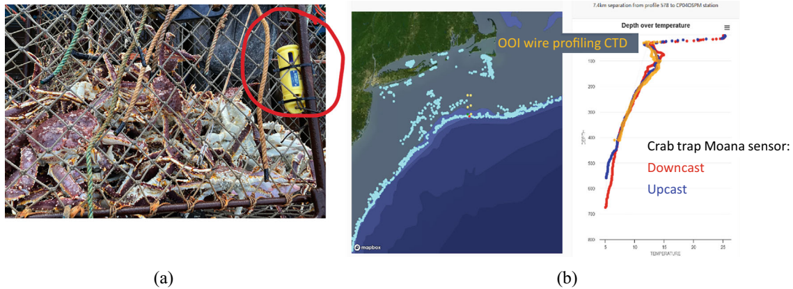
Fig. 3 ZebraTech Moana TD1000 sensor operating off New England, USA: a Moana TD1000 sensor (red circle; the yellow cage protects the sensor for mechanical impacts) installed in a crab trap; b temperature profiles measured by the Moana TD1000 sensor (red and blue lines) and by the wire-following CTD profiling of the U.S. Ocean
