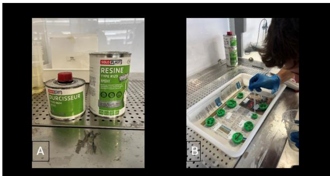
Figure 2: The two catalysts (a) and the preparation of the epoxy resin (b), which permitted the production of high-resolution casts from the already produced molds. Photographs taken by: Marina Lozano.
