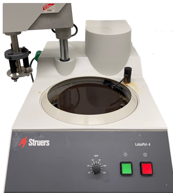
Figura 4. Máquina polidora (LaboPol-4, Struers A/S, Ballerup, Denmark).
