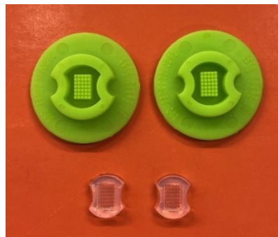
Figure 5.2 - Petri Dish 3D and respective agarose gel moulds.
