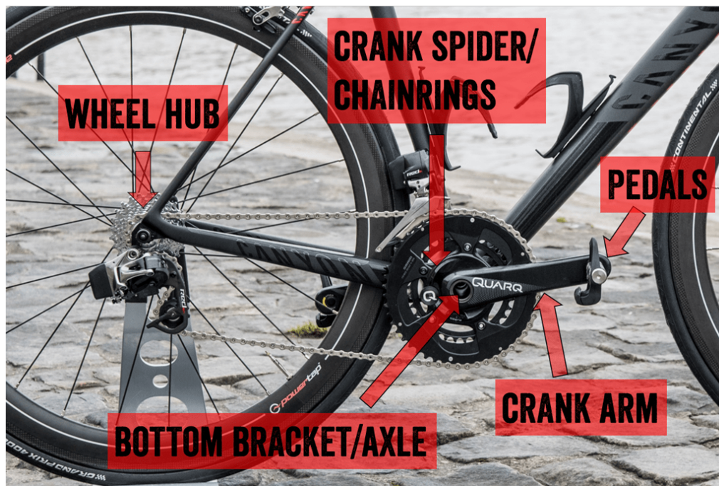
Figure 2.13: Power Meter Locations
