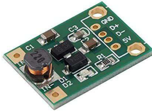
Figure 4.14: DC to DC Voltage Regulator
