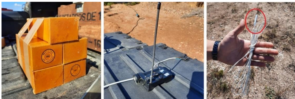
Figure 80 - Explosive Charge (5 kg of TNT) (Left), Blasting Machine (Middle), Detonator (Marked in red) (right)
