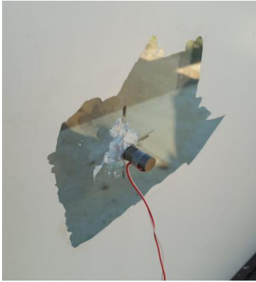
Figure 78 - Accelerometer glued to the glass
