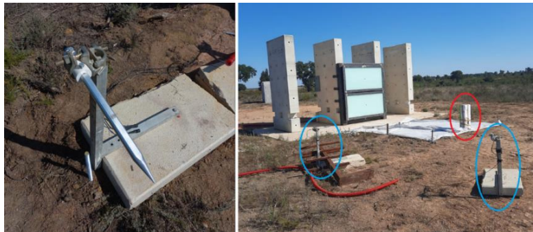
Figure 81 - Incident Pressure Sensor (Blue) and Explosive Charge (Red)
