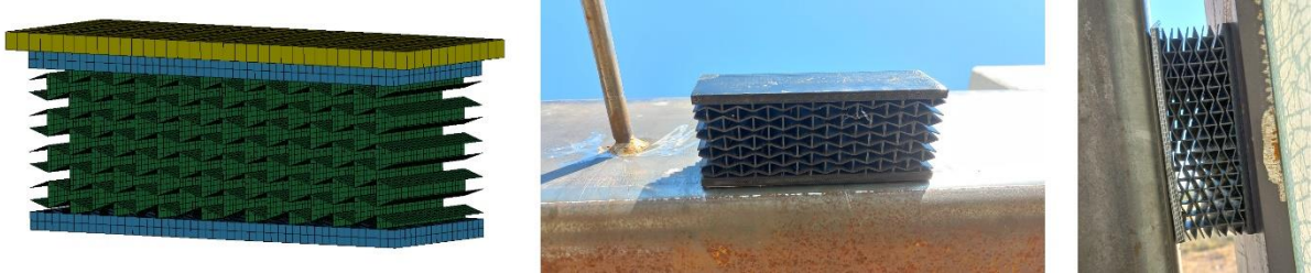
Figure 64 - FE Model of the dissipator (Left), Dissipator Glued to the Structure (Middle), Complete System of the structure (Right)
