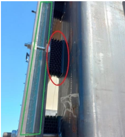
Figure 87 - Dissipator after charge of 5kg@9m (Red) and front glass plie broken (Green)
