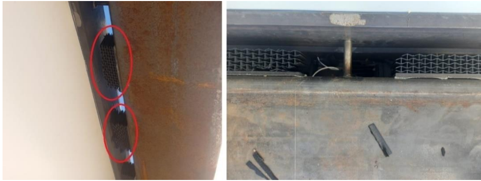
Figure 90 - Dissipator response to charge of 5kg@7m
