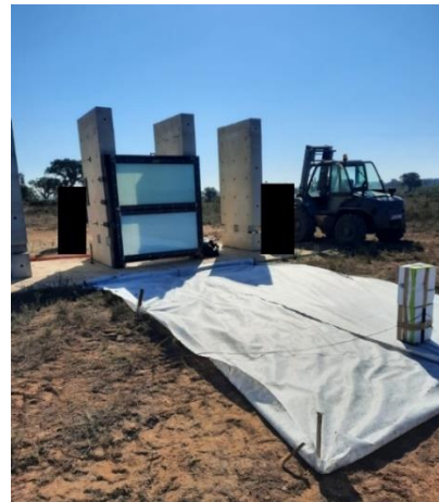
Figure 88 - Geotextile solution to prevent impacts on glass
