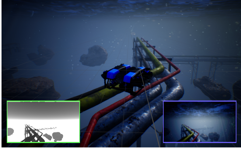
FIGURE 2.16: UNav-Sim example simulation. The bottom right displays the feed from a front-facing RGB camera, while the bottom left shows a corresponding depth image (Amer et al., 2023)
