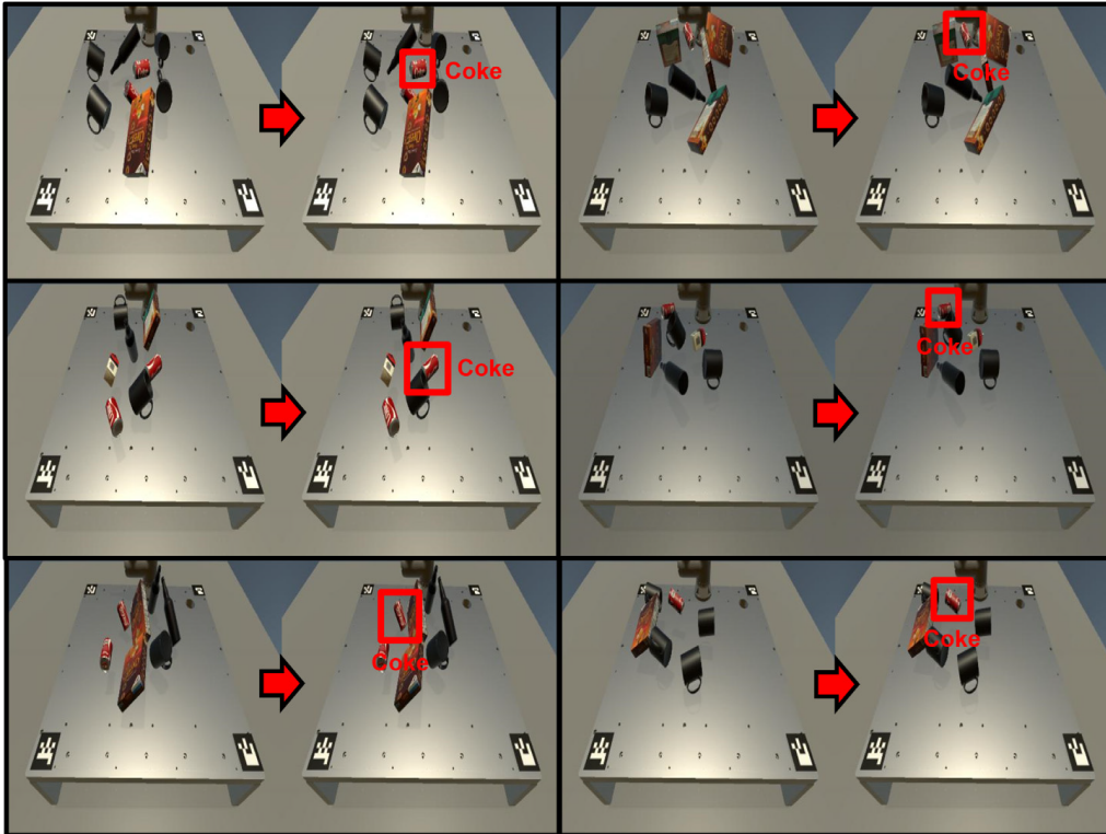
FIGURE 2.18: Synthetic data-based object detection training scene (Kim et al., 2024)
