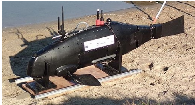
FIGURE 1.1: BUV 1 - Developed by the Polish Naval Academy (“Prezentacja finalna pojazdów SABUVIS”, 2018)
