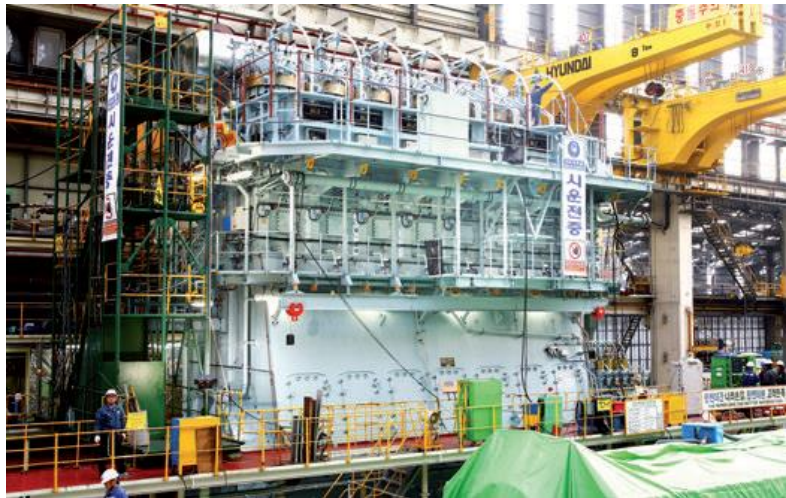
Figure 2.1 – 2-stroke low-speed Wärtsilä RT-flex 82T Diesel engine [16]
