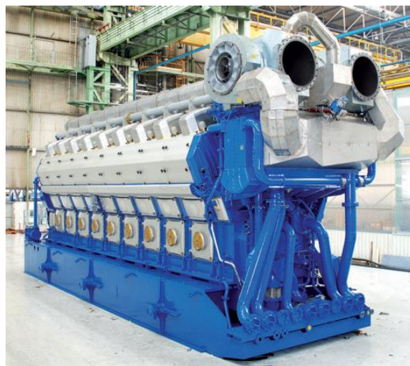
Figure 2.2 – 4-stroke medium-speed Wärtsilä 50DF engine [16]
