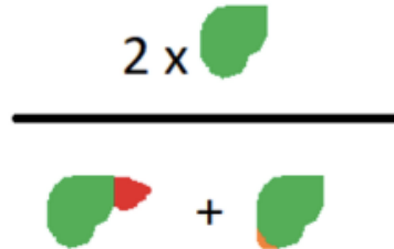
Fig. 1.5 Illustration of the calculation of DSC, with TP in green, FN in red, and FP in orange
