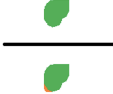
Fig. 1.4 Illustration of the calculation of precision, with TP in green, and FP in orange
