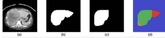
Figure 1: Illustration of Image Segmentation results: (a) Original image; (b) Ground truth segmentation; (c) Automatic segmentation; (d) Classification outcomes.
