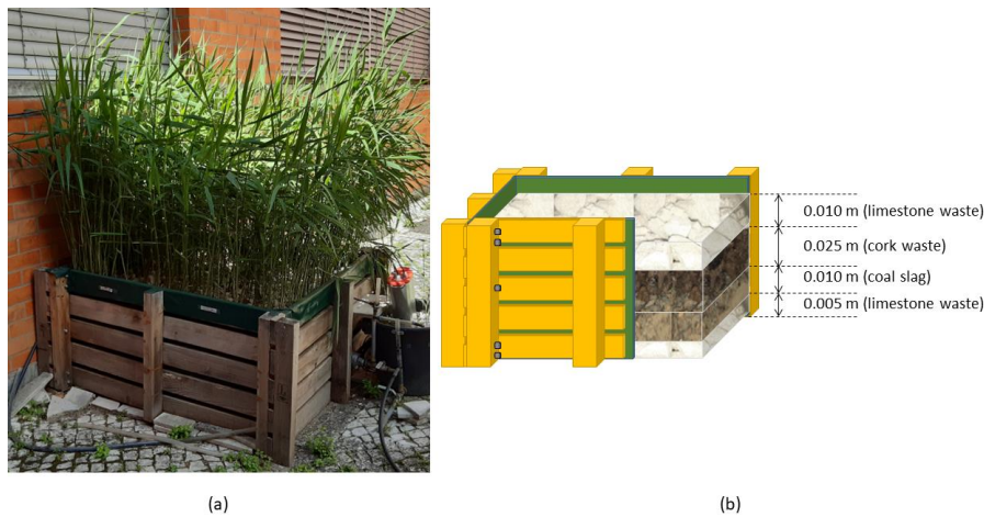
Fig.1. Picture of the CW prototype (a), and schema showing the filling media consisting in four layers of three recovered solid wastes (b).
