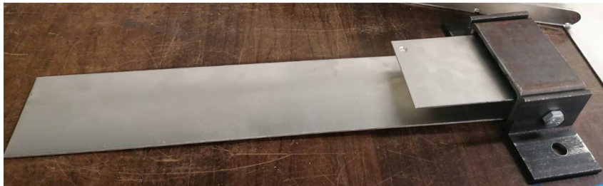
Figure 4.4: U-shaped dissipative flat bar bending device (UFBD) used for the experimental campaign.
