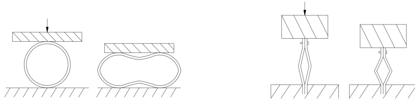
Figure 3.13: Experimental test on type I and type II specimen before and during deformation (Adapted from [9]).
