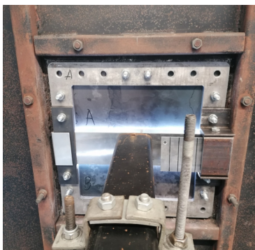
(a) UFBD configuration before the blast
