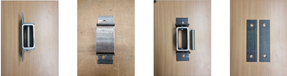
Figure 4.2: Details of the mechanism box and the two rectangular pieces of steel.
