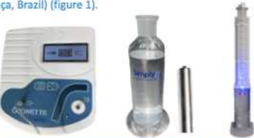
Figure 1 – Ozone generator machine; Ozone water bubbler system; Microbubble water ozonation column
