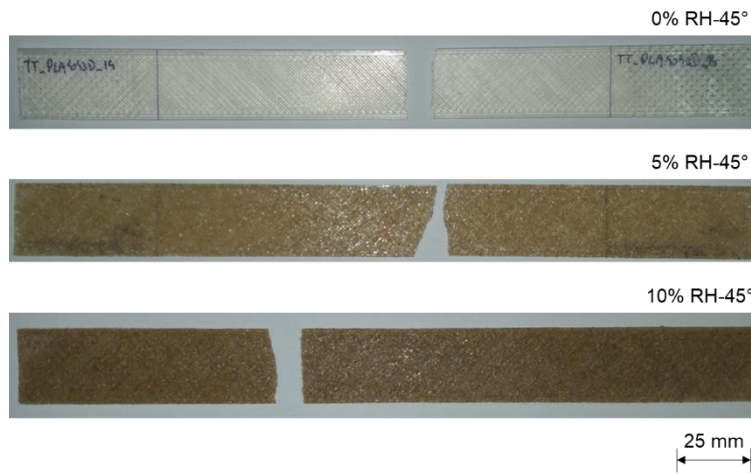
Figure 68- Tensile test fractured specimens printed at 45°.
