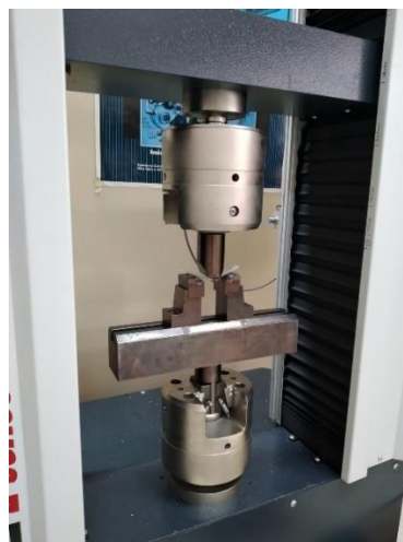
Figure 50- Impact® E-Series - TS 300 testing machine, flexural test assembly.
