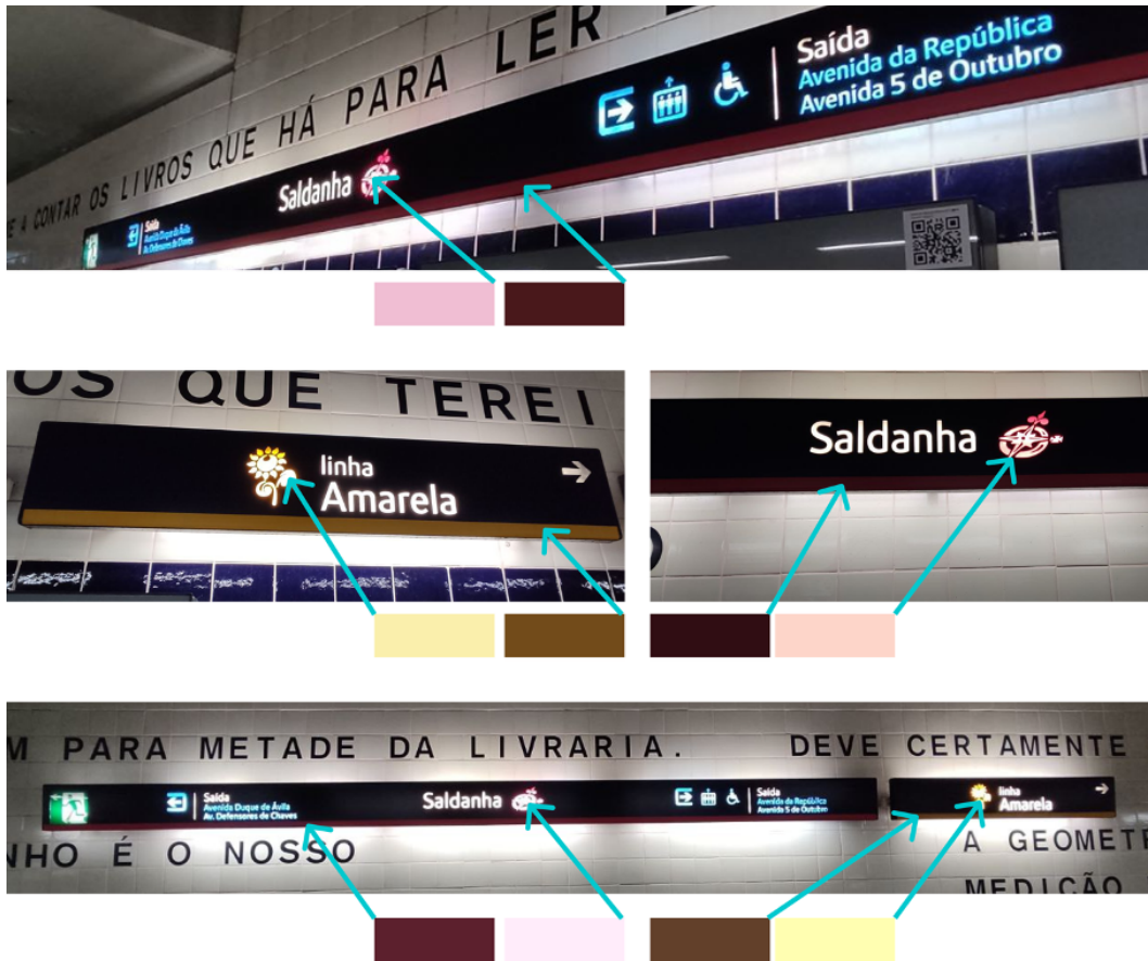
Figure 60. Example of interior sign lighting. Use of lightbox in signs and incorrect display of colours in the Lisbon Metro. All photographs in this collage were taken by the author, 2025.
