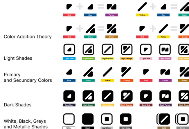
Figure D10: ColorADD code system for colorblind users. Adapted from ColorADD,n.d., https://www.coloradd.net/en/coloradd-code/ . © ColorADD.
