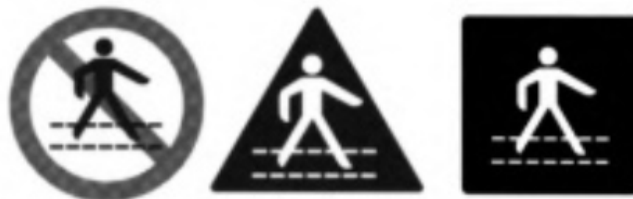
Figure 24. An example of how the same glyph, when combined with different shapes and colors, can change its meaning. From Wayfinding: People, Signs, and Architecture (p. 146), by P. Arthur & R. Passini, 1992, McGraw-Hill Book Company.
