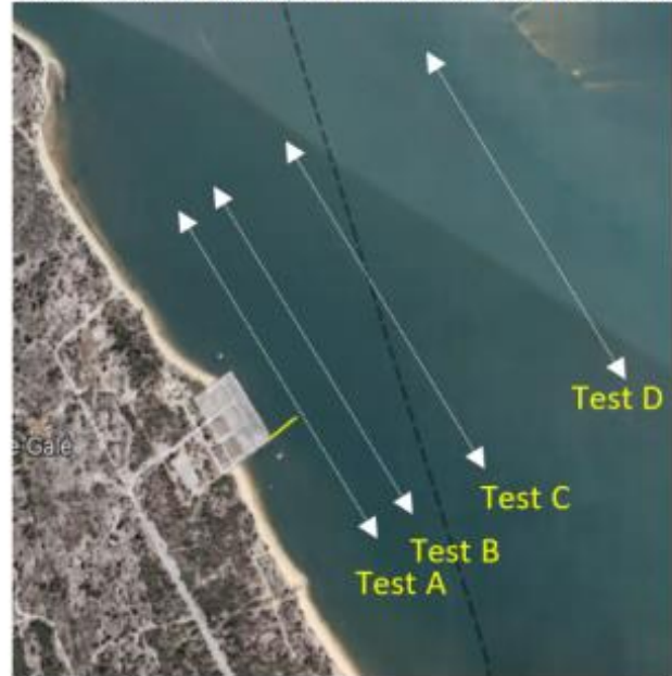
Fig. 9. Tests performed during the exercise to collect acoustic data: Test A - 100 yards, Test B - 200 yards, Test C - 400 yards, and Test D - 800 yards.
