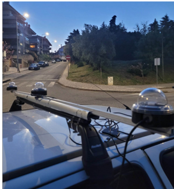
Figure 5.19: LX-GPS installed in a vehicle
