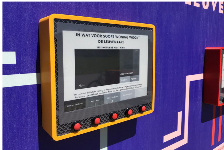
Figure 3. One of the polling devices in Citizen Dialogue Kit. The device displays the question in the top, the visualization of collected data (graph) in the middle, and has push-buttons in the bottom for each answer. Source: Cornelissen (2021).
