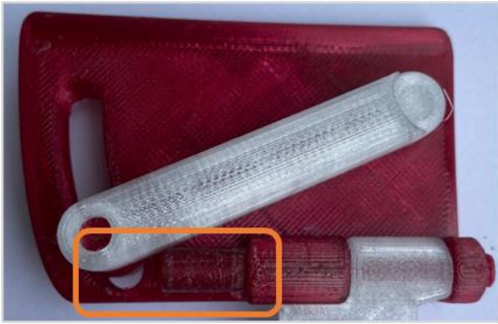
Figure 18 – Mandible Support's Reduced Angle Adjustment
