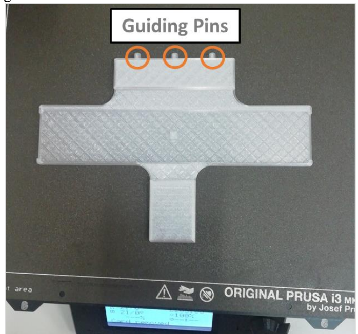
Figure 14 – Lower Part of the Main Back Portion Printed
