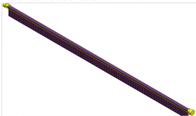
Figure 11 – Assembly of the Sliding Element and the 450 Small Elements
