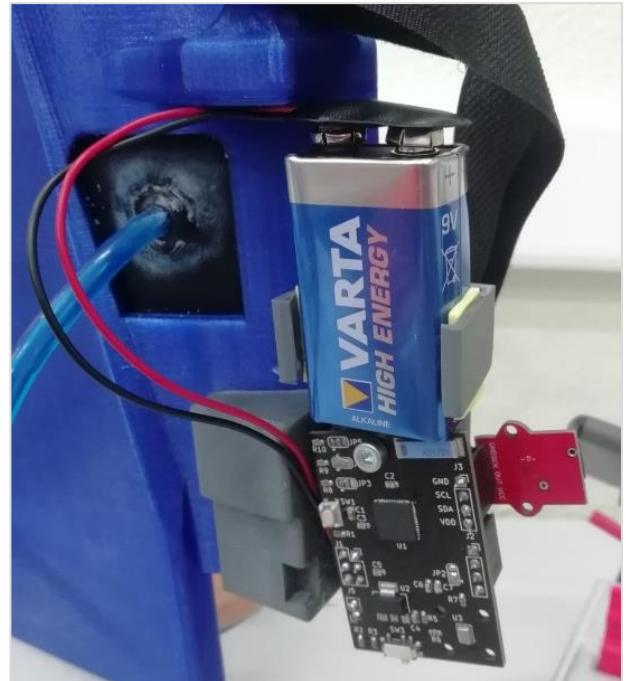
Figure 110 – PCB and Battery Integrated on the Collar
