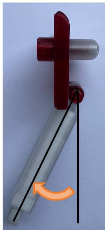
Figure 16 – Rotation Angle Between Mandible Support and Shoulder-Mandible Element
