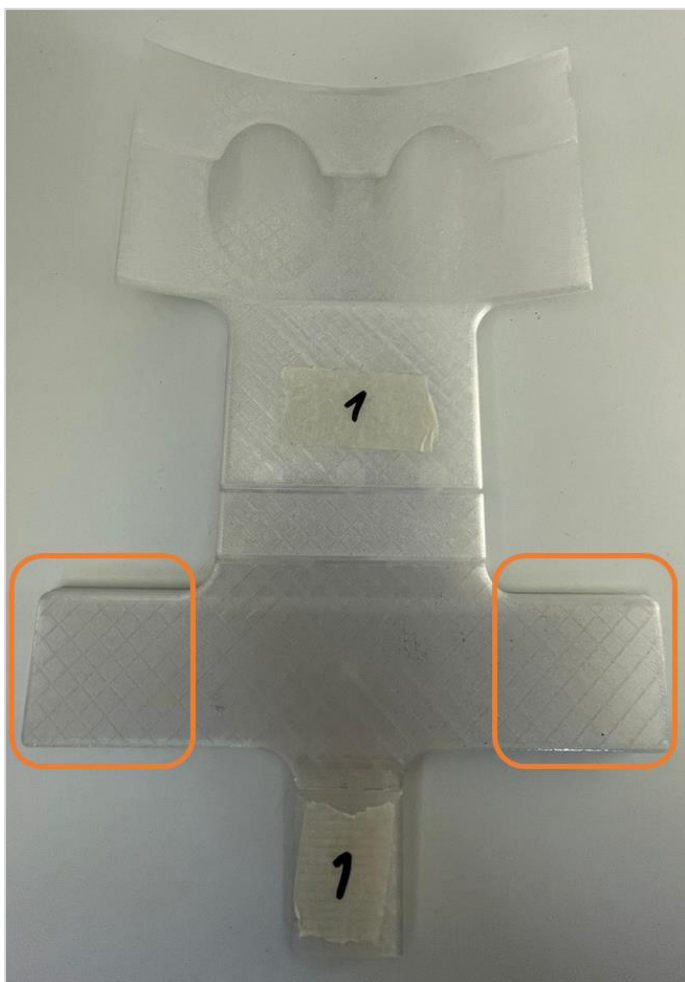
Figure 15 – Main Back Portion Assembled with the Loose Regions Signalled with Orange Contour
