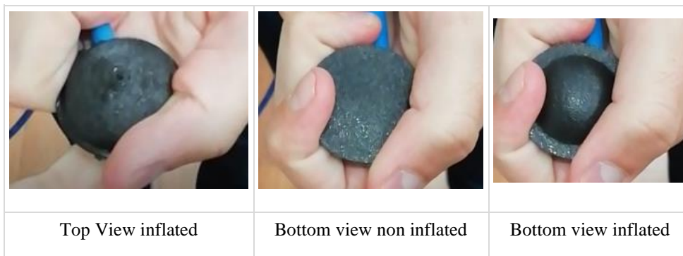
Figure 71 – Behaviour of Half Sphere-Shaped Balloon Inflated with Pressurised Air
