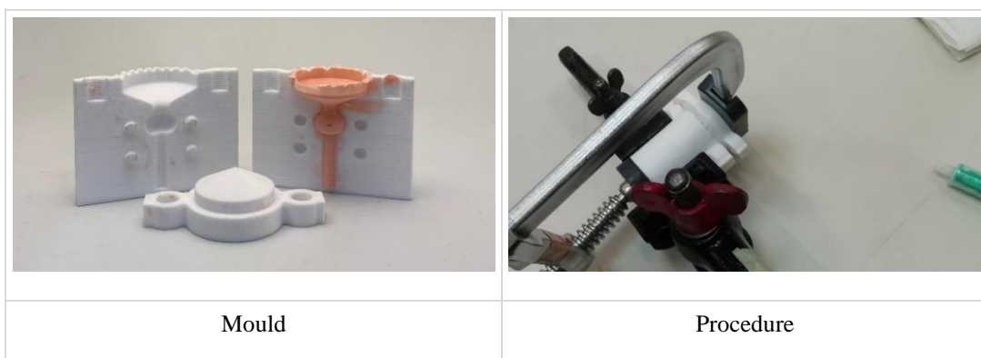
Figure 80 – Mould and Procedure for Producing the Silicon Cover
