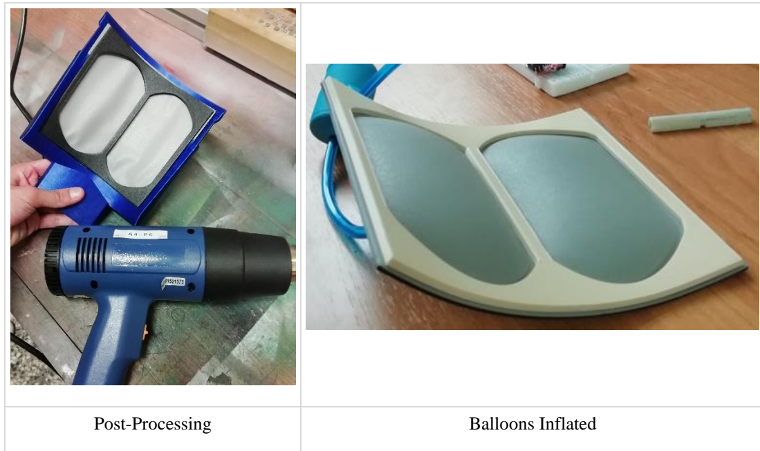
Figure 78 – Post-Processing and Test of the Balloons
