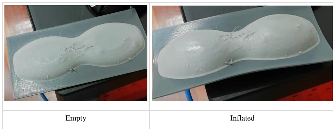
Figure 73 – Test of the Balloons with Rigid Base
