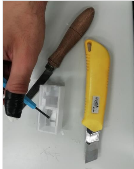
Figure 70 – Post Processing of One of the Shoulder Support Parts
