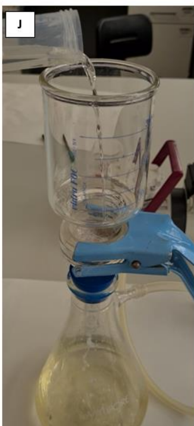
Figure 9 : Pictures of the extraction protocol of pollen and NPPs describe in Annex 1 (Goeury et De Beaulieu, 1979 ; Burjachs et al., 2003). F. Centrifugation G. Decant of KOH H. Water bath after removal of humic acids I. Flotation with Thoulet Liquor J. Filtering K. Removal filter and silica.
