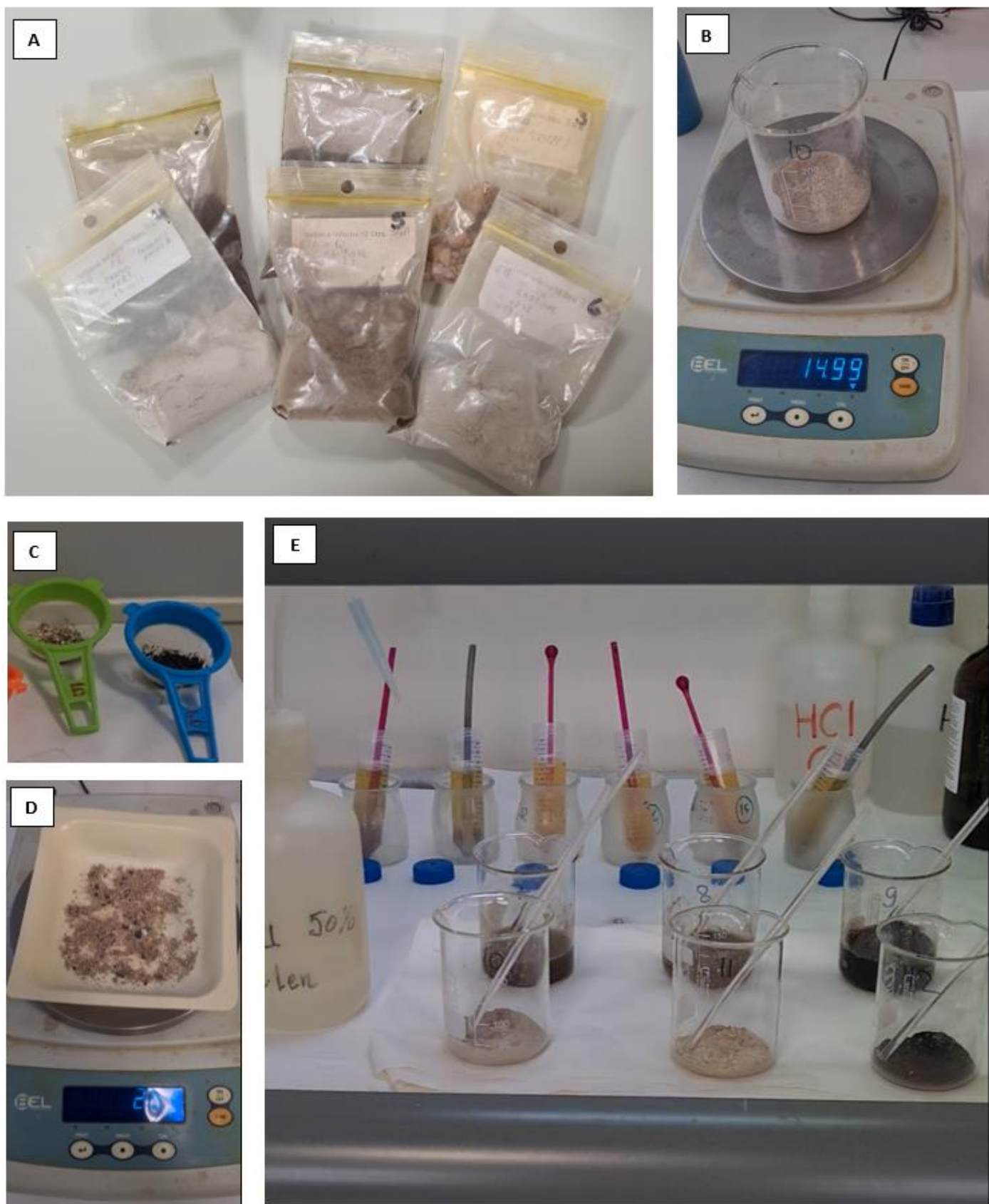
Figure 9 : Pictures of the extraction protocol of pollen and NPPs describe in Annex 1 (Goeury et De Beaulieu, 1979 ; Burjachs et al., 2003). A. Samples B. Sample Weight C. Sieving and D. Weight of coarse sedimentary E. Carbonate dissolution
