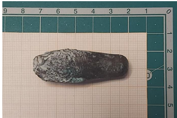
Figure 4.24: S3 recovered liner.
