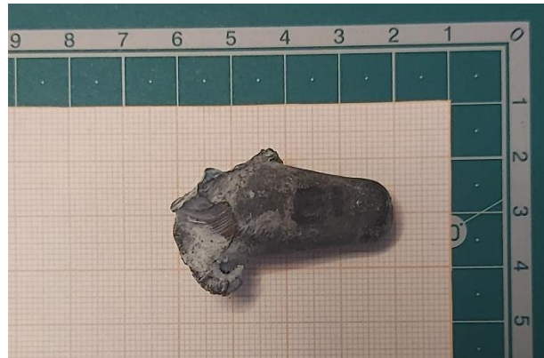
Figure 4.28: E1 recovered liner.
