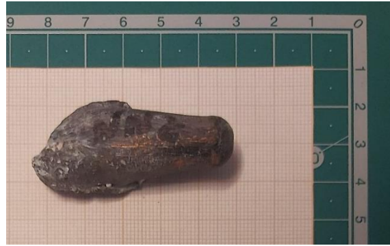
Figure 4.39: NN2 recovered liner.
