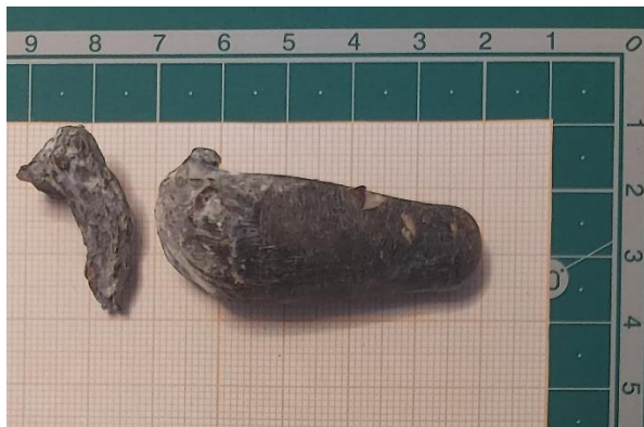
Figure 4.33: E3 recovered liner.
