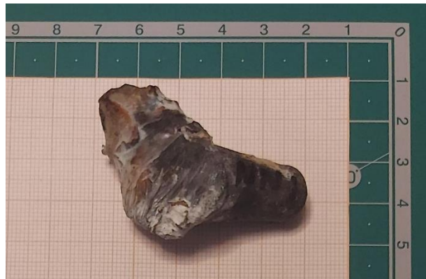
Figure 4.37: NN1 recovered liner.
