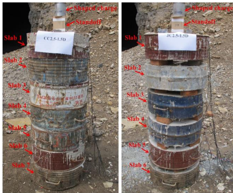
Figure 2.27: Layered and spaced concrete targets (Xu et al., 2020).
