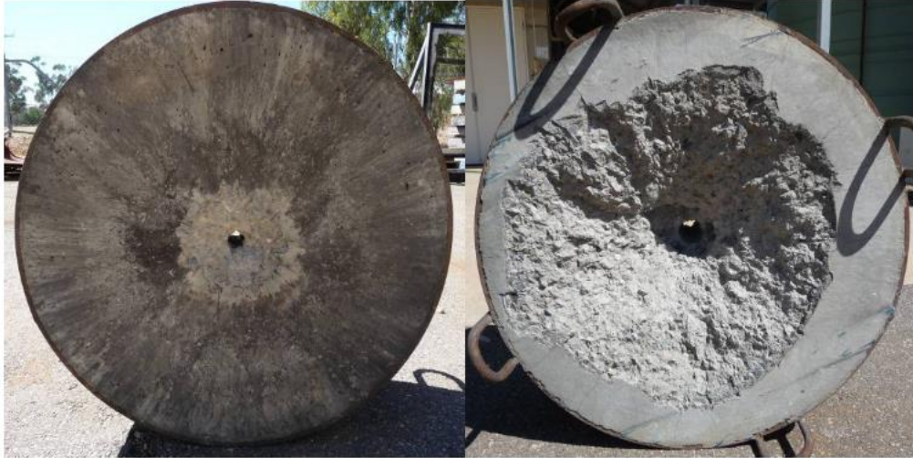
Figure 2.23: Plain concrete damage to front and rear face (Resnyansky et al., 2014).
