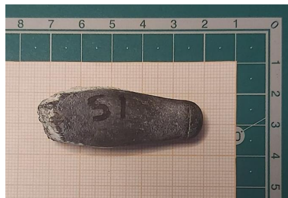
Figure 4.20: S1 recovered liner.
