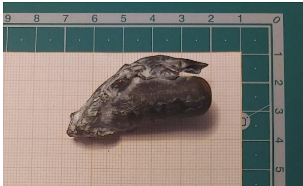
Figure 4.41: NN3 recovered liner.
