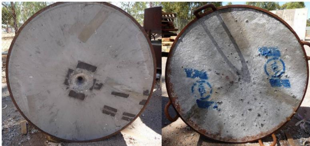
Figure 2.22: UHPC damage to front and rear face (Resnyansky et al., 2014).
