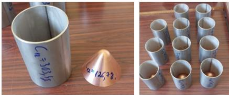
Figure 4.1: Copper liner and steel casing.
