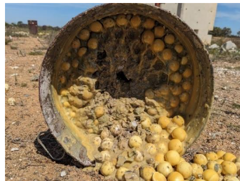
Figure 4.43: Spheres being held by the fluid.
