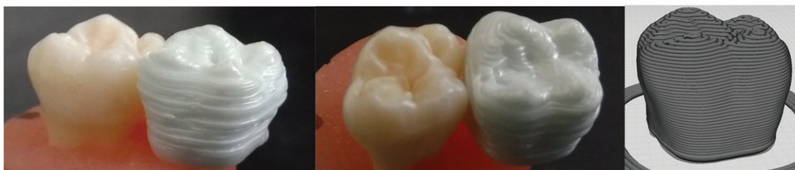
Figure 2. Post-sintering public domain molar tooth prototype printed using the using the 88 wt.% solid slurry next to an unrelated extracted tooth for comparison. The sliced 3D prototype tooth model used is shown in the rightmost picture.
