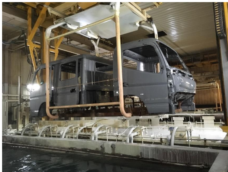
Figura 51- Hangar que desloca as cabines.
