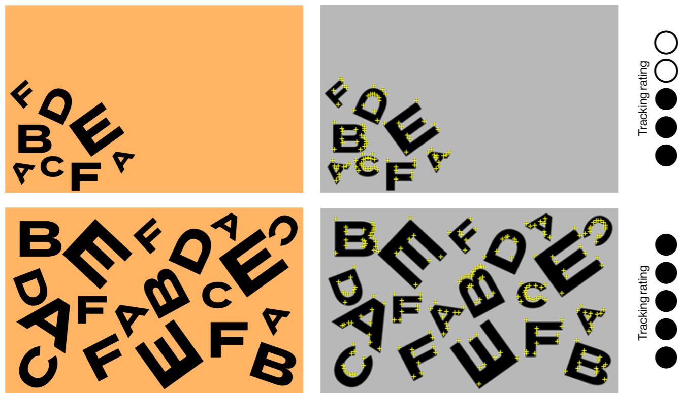
Fig. 18 – Target rating examples. The image below has more detail distributed among an even area, providing better results. Reference point maps and target rating retrieved from Vuforia Target Manager
