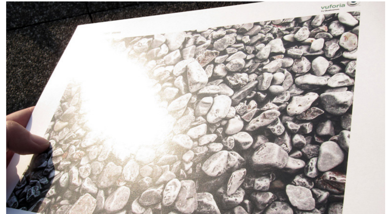
Fig. 22 – Glossy materials may generate undesired reflections that will occlude part of the image target. Retrieved June 5, 2019 from https://library.vuforia.com/
