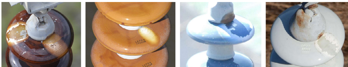
Figure 2.18: Flashover damages exemplification [31]
