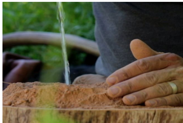
Figure 30: Preparation of clay dough. 1. Crushing the raw material 2. Grinding of the raw materials 3. Clay paste with water.
