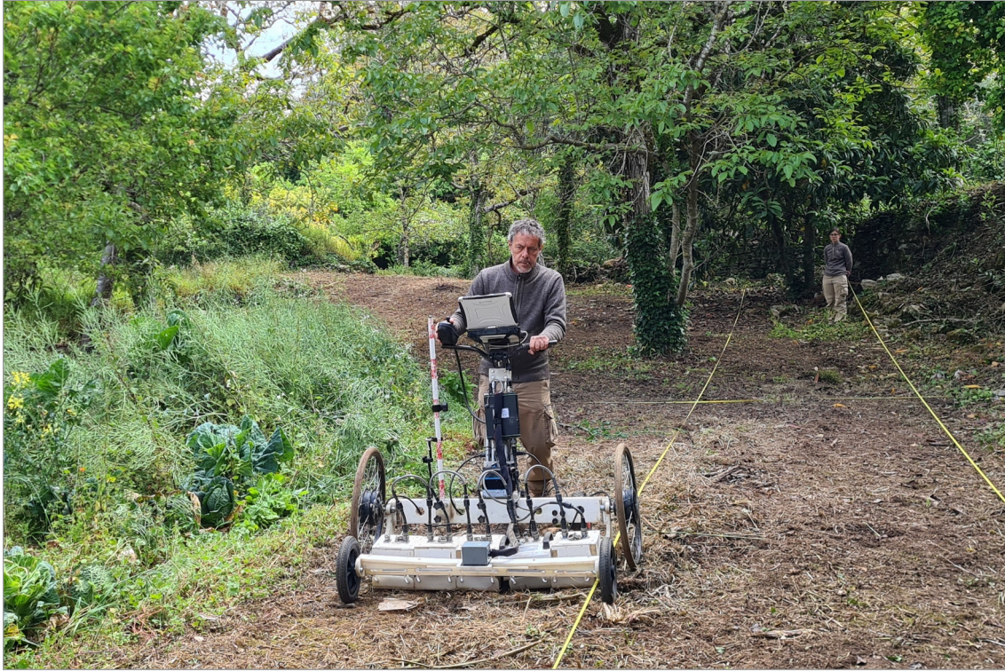
Figure 3: GPR measurements with IDS HI-MOD system in the Vale Norte (photo: Pedro Rodríguez Simón)
