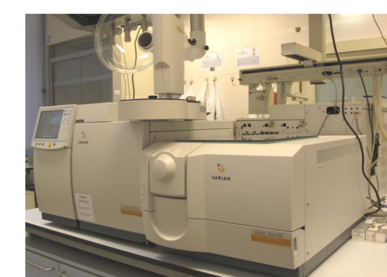
Figure 3 – GC-MS/MS: Bruker GC-450 GC coupled to a 300-MS TQD.
