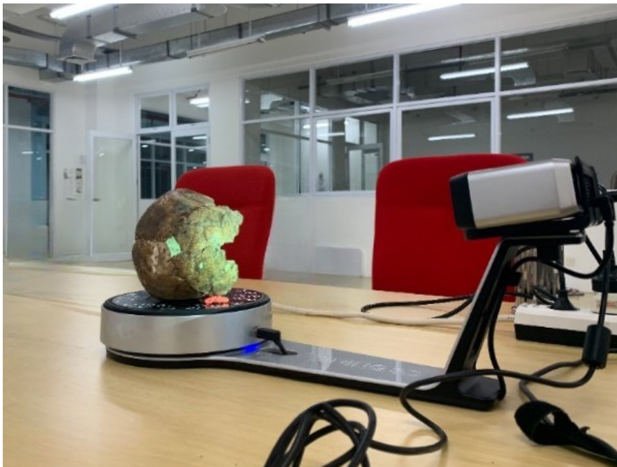
Figure 10. 3D scanning process using the Shining 3D EinScan-SP V2.
