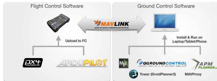
Figure 3. Options available for Flight Control Software and Ground Control Software (Retrieved from LambDrive, 2016).
