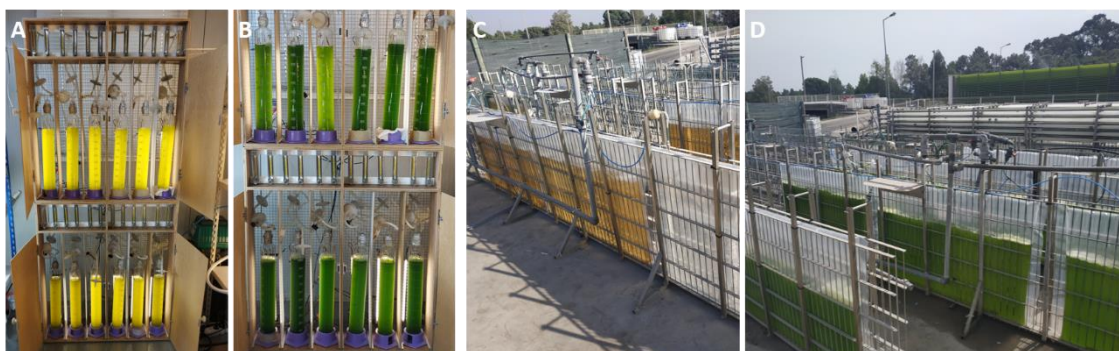
Figure 2.1 Laboratory-scale - bubble column reactors (1 L) with Chlorella vulgaris cultivation after inoculation (A) and a few days later (B). Pilot-scale - flat-panel reactors before inoculation (C) and after inoculation (D).
