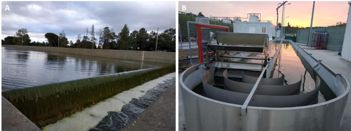
Figure 1.2 Thin-layer cascade system (A) and a pilot raceway (B) are the two open systems at Allmicroalgae facilities.
