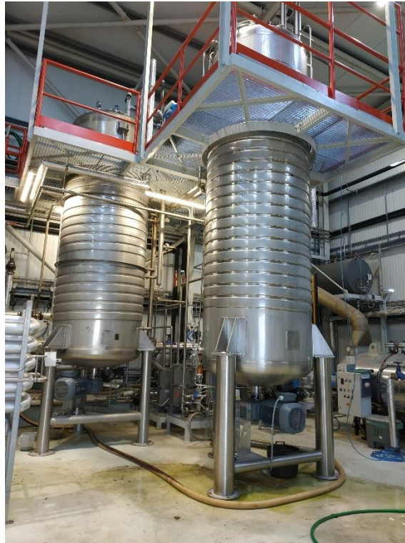
Figure 1.4 Allmicroalgae's industrial fermenters of 5000 L
