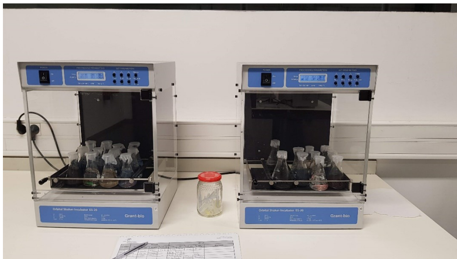
Figure 25 - Leaching assays in the Orbital shaker ES20 Grant-bio, for 15h at 30°C and 200 rpm.
