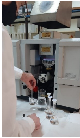
Figure 21 - Atomic Emission Spectrometer (AES), produce by Horiba model Ultima @ LNEG.
