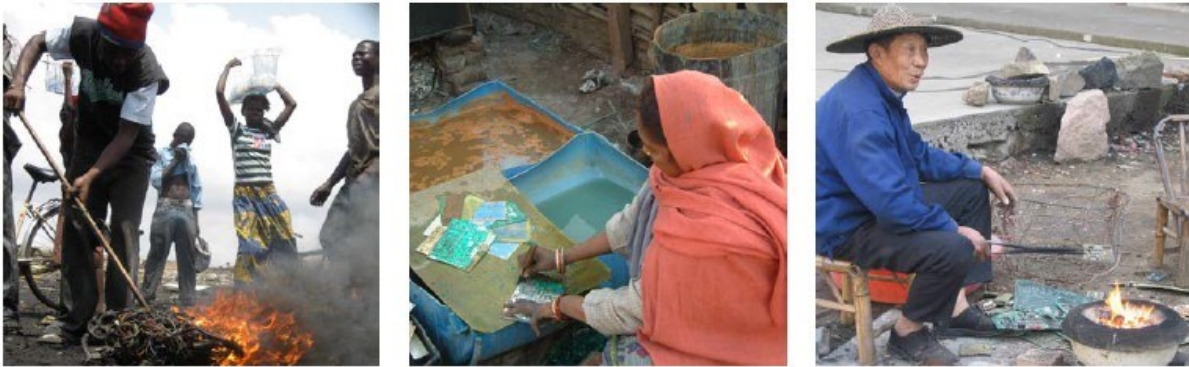
Figure 3 - Typical recycling processes applied in the informal sector of developing countries, adapted from [15], from left to right: open burning for copper recovery, hand pinking of components, burning for desoldering of PCBs.
