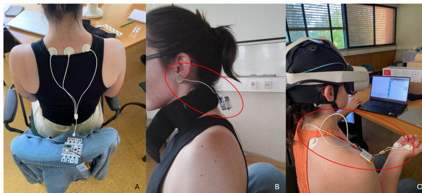
Figure 3.5: (A) ECG sensors placed over the C7 vertebra and the trapezius muscle; (B) EDA sensor on the earlobe; (C) EDA sensor placed on the palm of the hand.
