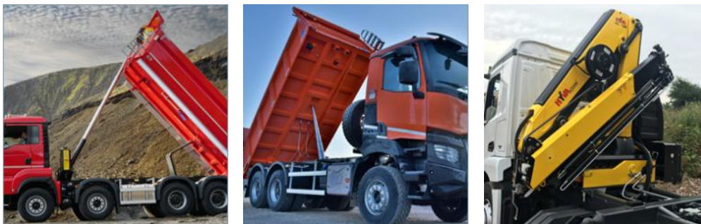
Figura 6 - Front-End Cylinders, Underbody Cylinders e Truck-Mounted Cranes
