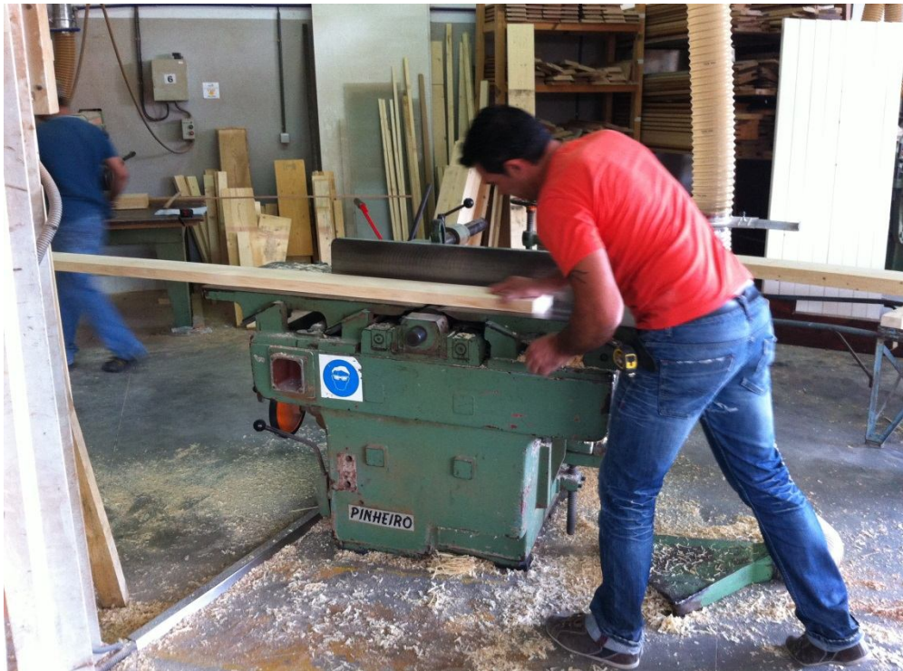
Fig.5 – Falta de EPI's.
