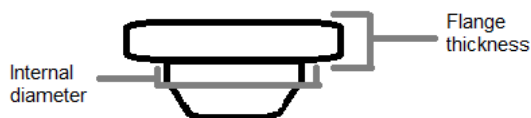
Figure 5 - Representation of the measurements taken for the rubber stoppers used in Hikma.
