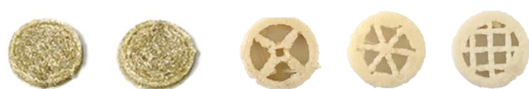
Figure 2. Typical FDM 3D-printed tablets with simple and complex geometries
