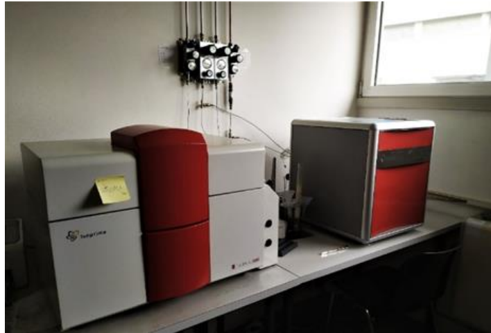
Fig. 4.7. 1, The photo of the EA-IRMS instrument. The right part is the 'Elementar Vario Microcube' elemental analyser, and the left part is the ' ISOPRIME 100 IRMS' mass spectrometer
