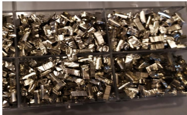
Fig. 4.7. 2, The photo of tin capsules used for IRMS analysis
