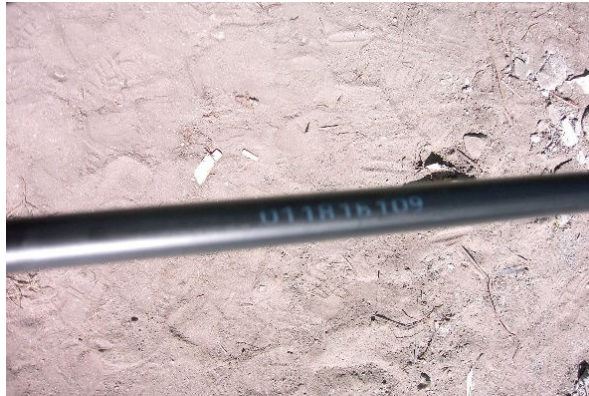
Figura 4.5: Cabo Aerial Cable 15 kV.
