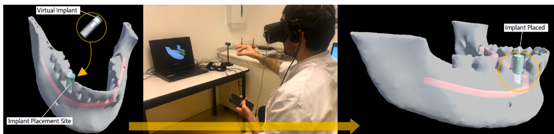
Fig. 7. Participants were asked to place a virtual implant at a specific bone-loss area location within a subject-specific 3D model of a lower jaw.
