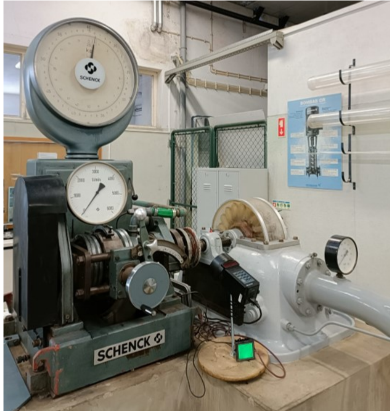
Figure 6.4: Equipment available at the LHM of ISEC for \dot{W}_{shaft} measurement.
