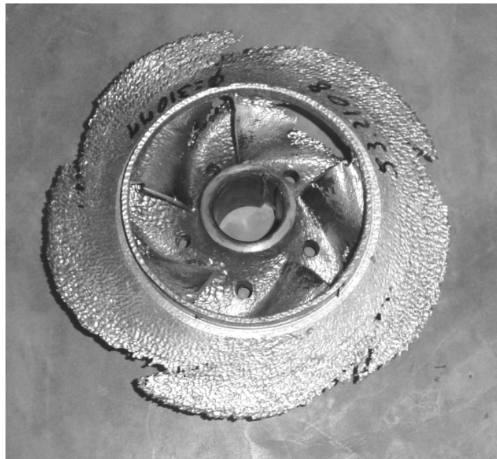
Figure 3.5: Destructive effects of cavitation on a pump impeller.
