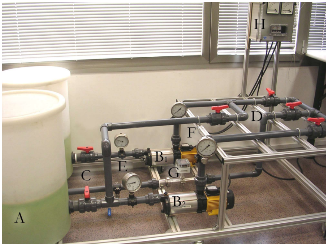
Figure 4.3: Centrifugal pump test bench for series and parallel configurations, including instrumentation, at the LHM of UMH.
