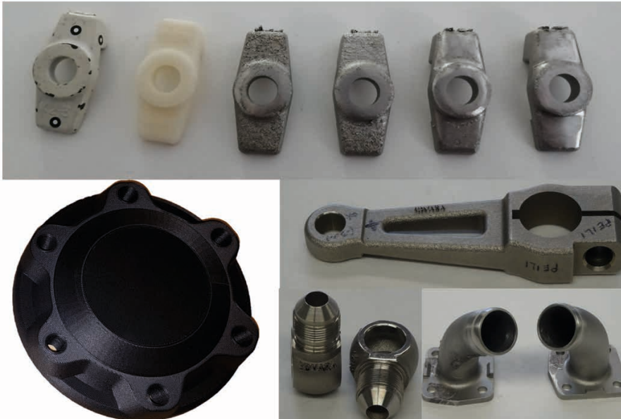
Figure 3 – Additively Manufactured spare parts (polymer and metal) to Mechanized Battalion Armored Personnel Carrier (APC)
